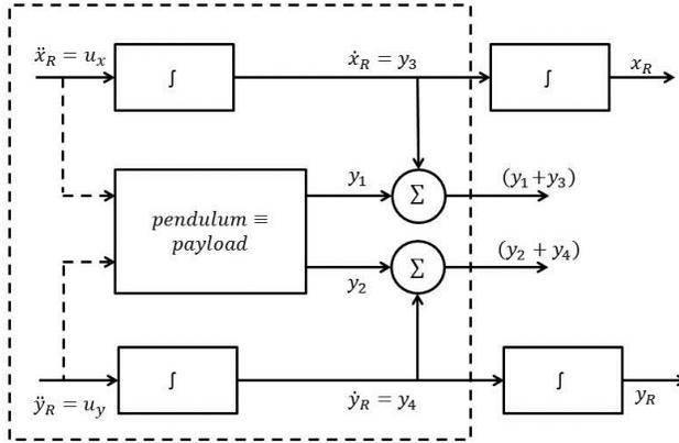
Fig 2: Spider crane as interconnection of passive systems
